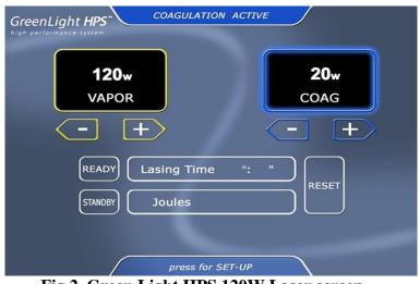
Fig 2 .Green Light HPS 120W Laser screen
